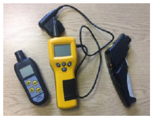
Selection of some of the tools a surveyor should have at their disposal, such as hygrometer, moisture meter and surface thermometer.
