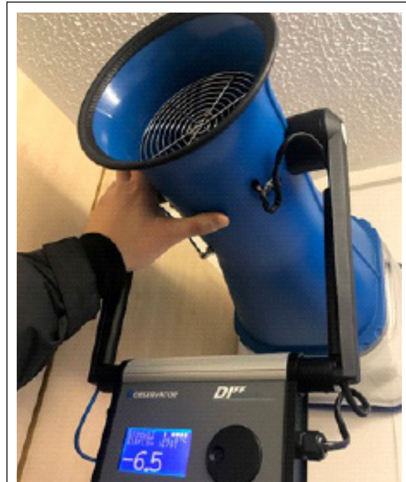
Unconditional method of testing a type 1 ventilation system using a powered hood.
